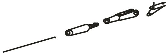
The rudder is mounted on clip-on hinges. Cut out the notches for rudder hinges with a razor blade, insert the hinges inside, fixing them with a lean instantaneous cement. Clip the rudder to hold.
